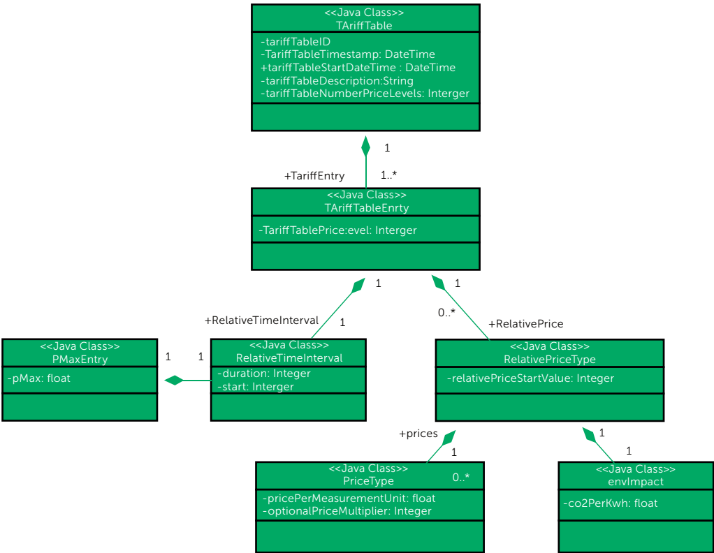
FIGURE 11.9 | CLASS DIAGRAM OF VARIABLE ELECTRICITY PRICE
