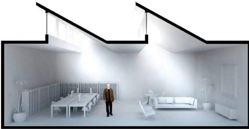
FIGURE 4.6.2 | TYPICAL SAW-TOOTH ROOF LIGHT DAYLIGHT HARVESTING
