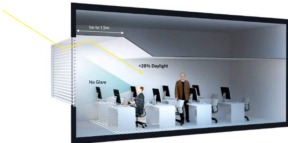
FIGURE 4.5.7 | DAYLIGHT ILLUMINATION LEVEL IS 28% HIGHER THAN FIGURE 4.5.6
