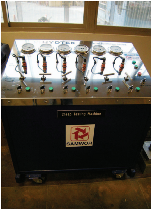
Hydraulic system driven by air compressor
