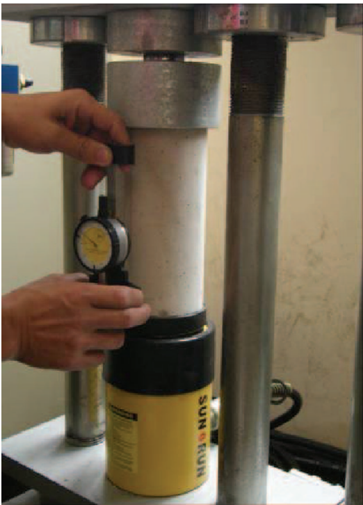
Taking measurement after loading with Demec gauge
