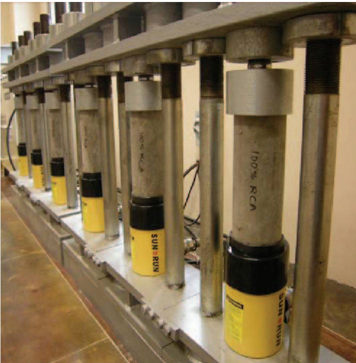
Metal frame for specimen loading
