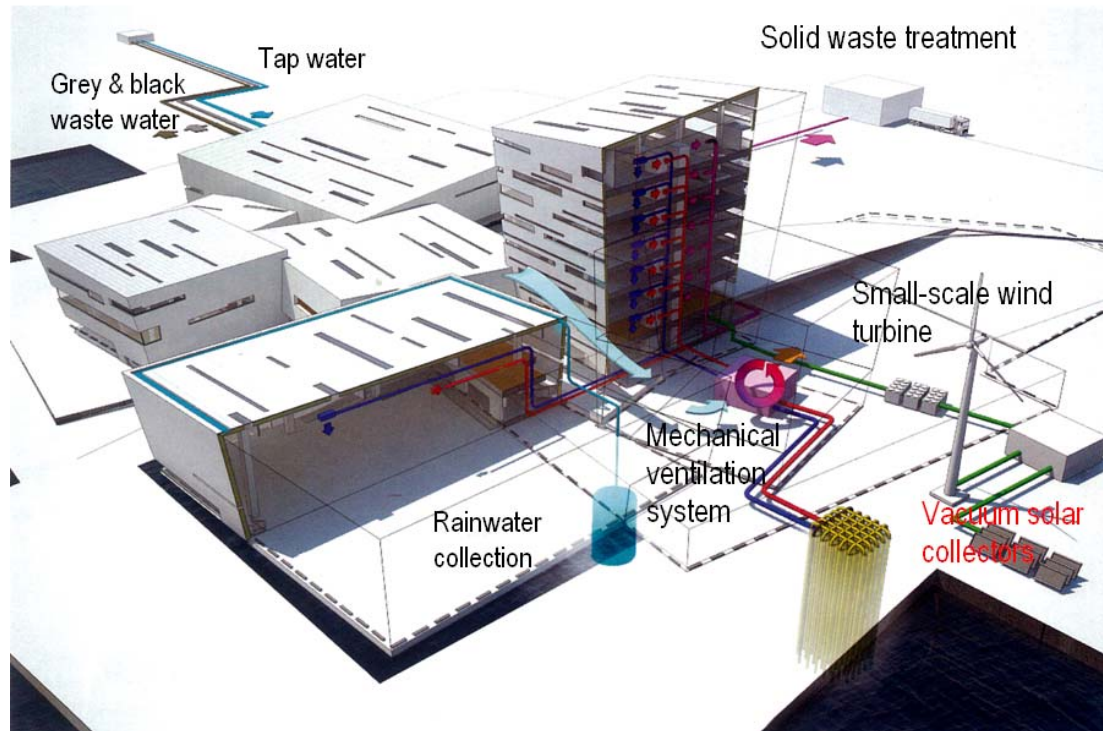
Figure 13 technical systems for a climate-neutral building in Sustainability Centre contain mechanical ventilation system, borehole system, wind turbine and vacuum solar collectors (Hessle, 2009, p. 81).
