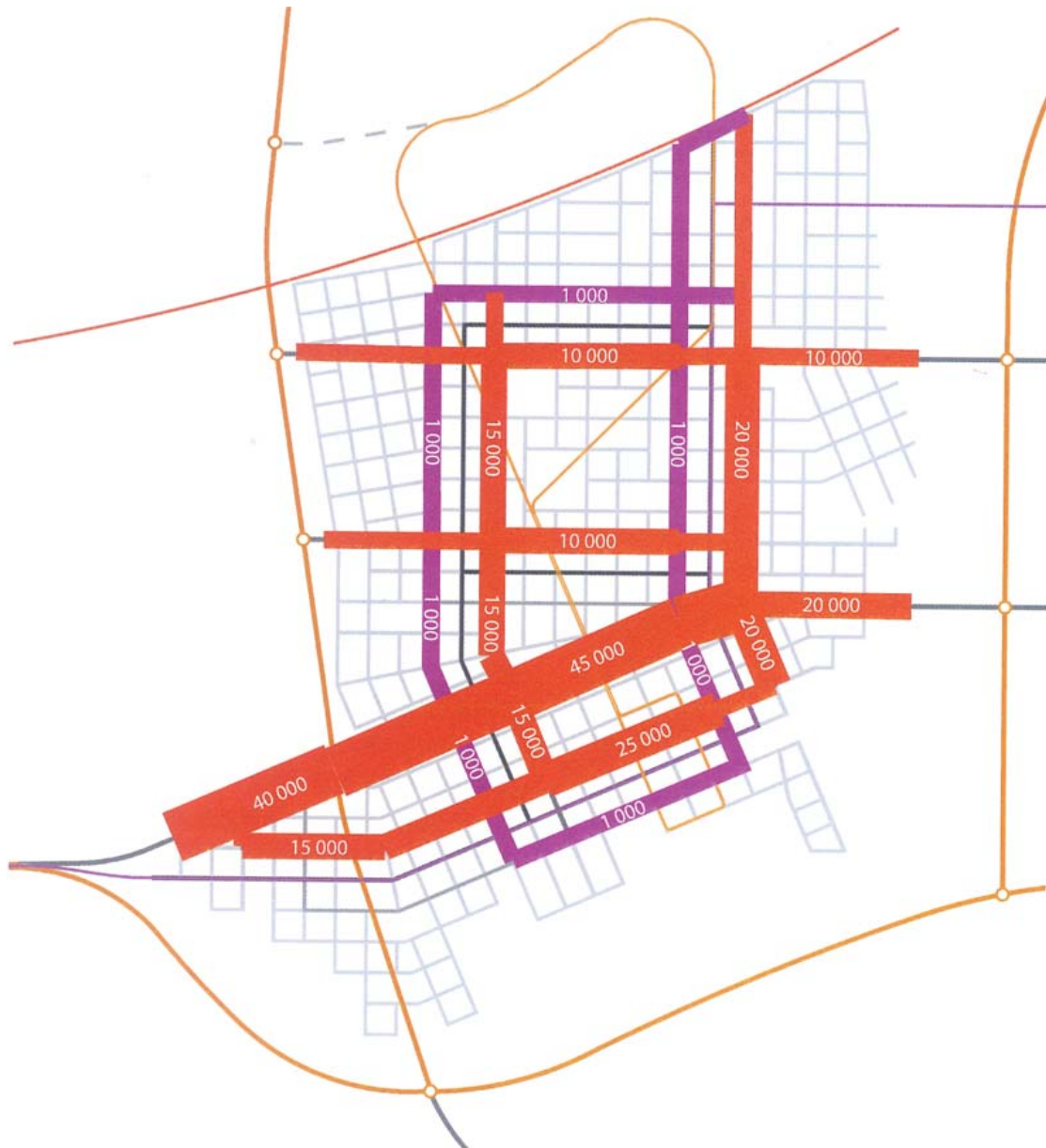
Figure 54 the illustration shows the estimated daily number of travelers by public transportation in 2030. The red lines are the estimated daily number of travelers by BRT. While the purple lines are the estimated daily number of travelers by light rail system (Joachim, 2009).
